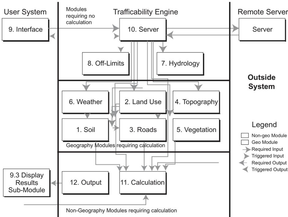
Figure 1: Architecture of the Trafficability Engine
