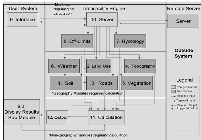
Figure 1: Architecture of the Trafficability Engine
