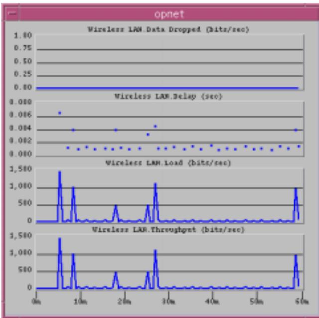
**Figure 3.** Typical Network Data Available from OPNET
